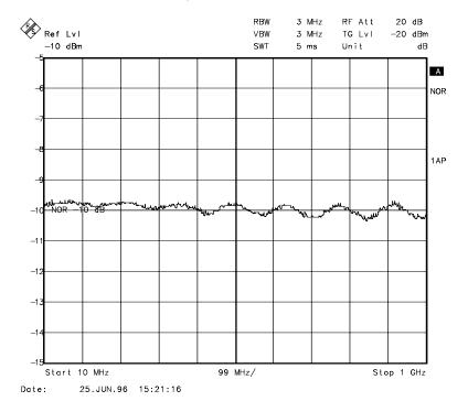
Fig. 2.13-1 Measurement of a 10dB attenuator pad with 1 dB / Div
