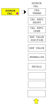
The *SOURCE CAL softkey* opens a submenu comprising the calibration functions for the transmission and reflection measurement.
