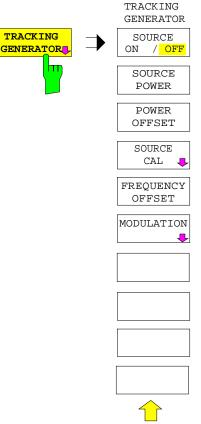
The *TRACKING GEN* softkey opens a menu for setting the functions of the tracking generator.
