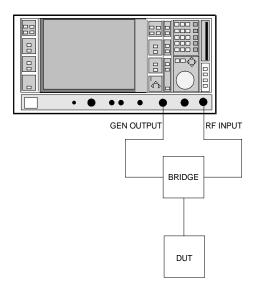
Fig. 2.13-6 Test setup for reflection measurements
