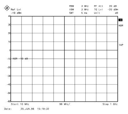
Fig. 2.13-5 Measurement with REF VALUE 20 dB and REF VALUE POSITION 50%
