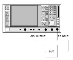
Fig. 2.13-1 Test setup for reflection measurements
